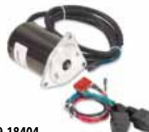
9-18404 Power Trim Motor Replaces: Yamaha 6G5-43880-00-00, 6G5-43880-01-00 Fits: 115-225hp 1987-91 Converts original 3-wire motor to a 2-wire High performance motor. Includes harness/relay kit, and o-ring, 3-bolt mount Important! 68.3mm mounting flange, 2mm thick shaft blade thickness
