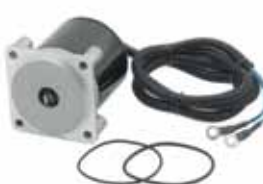
9-18305 Power Trim Motor Replaces: Suzuki 38100-99E01-OEP, 38100-95E01-OED Fits: DF60/70 1998-2000, DT65/75 1995-97, DT85 1995-2000, DT115/140 1996-2001 2-wire, 2-bolt mount
