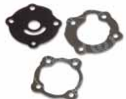
9-43406 Wear Plate w/gasket Replaces: Johnson/Evinrude 329391 Fits: 25 hp, 1979-84
