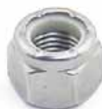
9-72003 9-72003-10 (Bulk Pkg 10) Nut, Stainless Steel Nylock Replaces: Mercury 11-45592 Thread Size: 5/16 X 24
