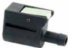
9-38011 Fuel Connector Replaces: Mercury 22-13563T7 3/8" hose barb
