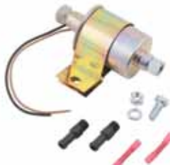
9-35436 Fuel Pump, Electric Universal Applications 12V 5-9 PSI @ 16.8 GPH 1/8" Female Pipe Thread
