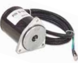
9-18407 Power Trim Motor Replaces: Yamaha 6H1-43880-02-00 Fits: 50-90HP 1992-95, 40HP 1994, 70-90HP 1996, 60/70/90HP 1997 - Up 2-wire connection, 3-bolt mount, o-ring included
