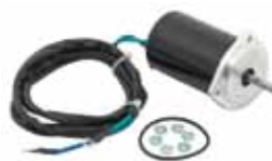
9-18409 Power Trim Motor Replaces: Yamaha 62Y-43880-00 Fits: Late model 4-stroke applications 2-wire connection, 3-bolt mount 1.5" shaft from seat to flat blade
