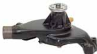
9-42604 Pump, Water Circulating Replaces: Mercruiser 850454-1, OMC 987447, Volvo 3855991, Crusader 30103, PCM RA057019 Fits: Big Block GM V-8 454 & 502 cid
