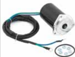
9-18401 Power Trim Motor Replaces: Yamaha 62X-43880-09-00, 62X-43880-01-00, 62X-43880-00-00 Fits: 40-100hp 1995-2003, 2-wire motor, 3-bolt mount, o-ring included
