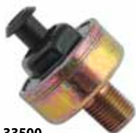
9-33500 Knock Sensor Replaces: Mercruiser 805544T / Volvo 3854512 Fits: MCM/MIE GM V-8 454, 502, 540, 572
