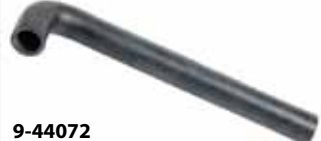
9-44072 Hose, Molded T-stat hsg to front of exhaust manifolds 1" (25mm) I.D. Replaces: Mercruiser 32-48132 Fits: MCM/MIE V-8 305, 327, 350, 427, 454 engines 1969-95
