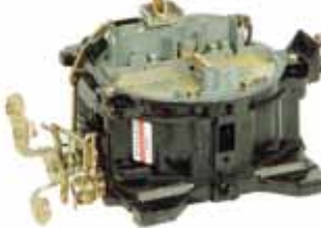
9-34008 Remanufactured Carburetor Replaces: Mercruiser 1347-8289A1 Fits: 4 bbl Rochester V-8 Engines
